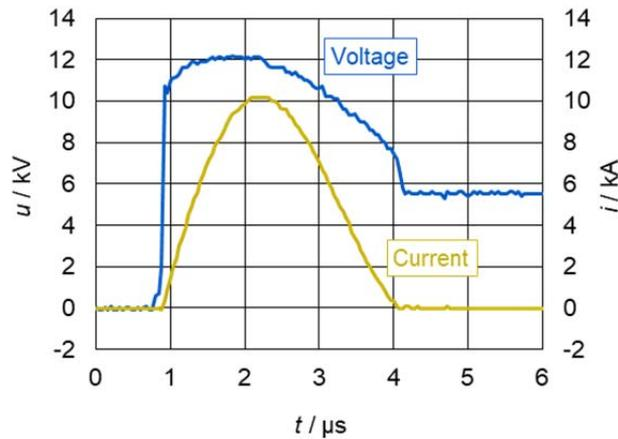
produced in a low-inductance, frequently coaxial test setup by a practically undamped capacitor discharge into the test sample. The current amplitudes are within a range of 1.5 kA to 20 kA. The oscillogram depicts an example of a residual voltage measurement on an MO resistor at a steep current impulse of 10 kA.
