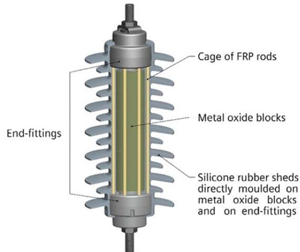
**Fig. 16:** Cross-sectional drawing of a polymer-housed MO distribution arrester
