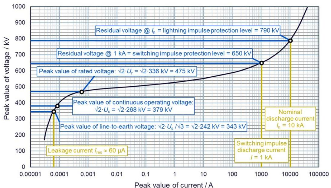
**Fig. 2:**  $U$ - $I$ -characteristic of a typical MO arrester ([class SM](#)) in a solidly earthed neutral 420 kV system
