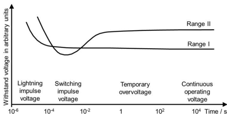
As a result, equipment in "range I" can be adequately characterized and qualified dielectrically by testing just with alternating and lightning impulse voltages, but tests with switching impulse voltages are mandatory for equipment in "range II" to cover the dielectric strength and to meet the minimum of the withstand voltage there.
