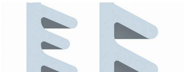
**Fig. 11:** Alternating shed profile (left) and normal shed profile
