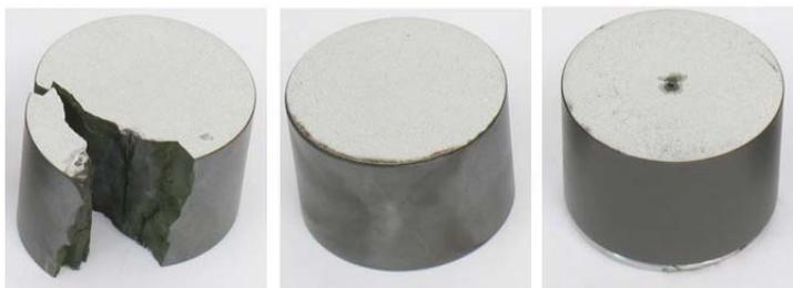
turing, or flashover of the MO resistors may occur (see picture). Up to IEC 60099-4 Ed. 2.2, the energy handling capability was only defined by the →[line discharge class](#). With IEC 60099-4 Ed. 3.0 new energy handling definitions have been introduced. The single energy handling capability is now specified by the →[repetitive charge transfer rating](#) ( $Q_{rs}$ ). The single impulse energy handling capability is smaller than the →[thermal energy handling capability](#).
