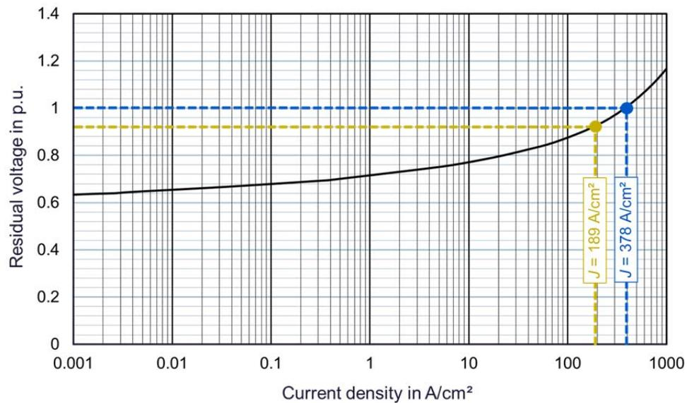
**Fig. 23:** *E-J-characteristic* derived from the *U-I-characteristic* of Figure 2
