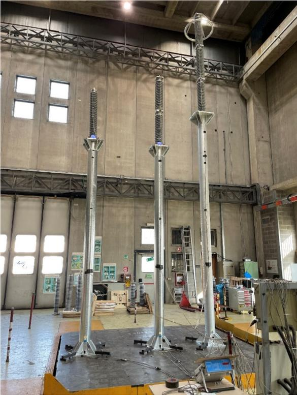
**Fig. 24:** Polymer housed arresters for system voltages of  $U_s=170$  kV,  $U_s=245$  kV and  $U_s=420$  kV during seismic testing on a shaking table
