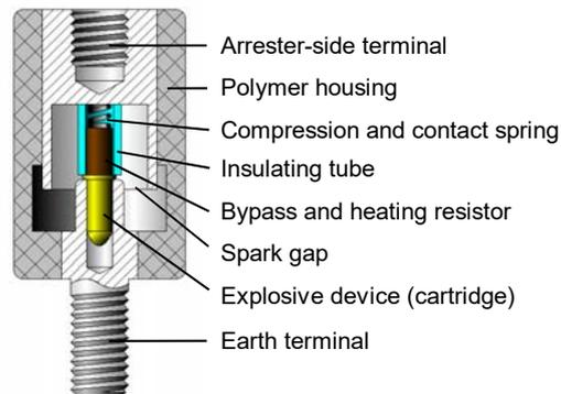
Principle drawing of a disconnecter triggered by an explosive device
