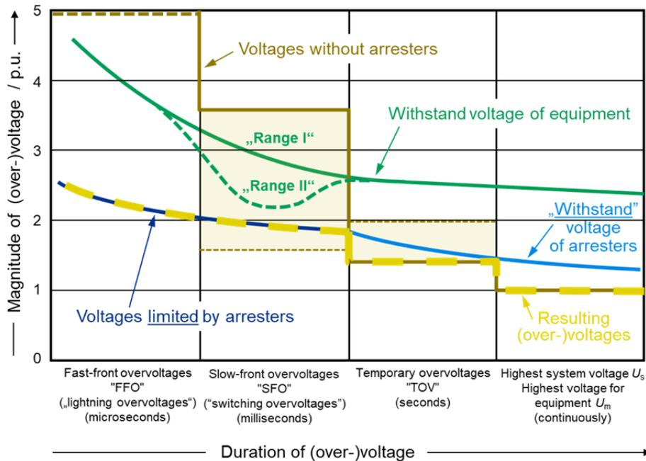
**Fig. 1:** Schematic representation of the magnitude of voltages and overvoltages in a high-voltage electrical power system versus duration of their appearance ( $1 \text{ p.u.} = \sqrt{2} \cdot U_s / \sqrt{3}$ )
