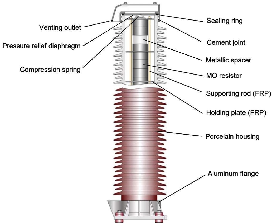
**Fig. 9:** Cross-sectional drawing of the unit of a porcelain housed MO arrester
