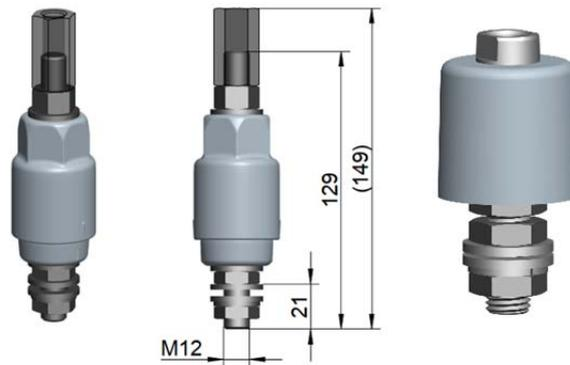
Disconnectors without pyrotechnics; left/middle: for distribution arresters;
