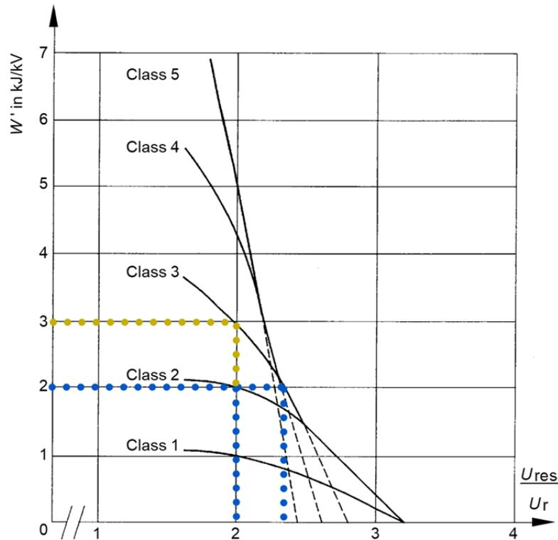
**Fig. 28:** Specific energy in kJ/kV of rated voltage dependent on the ratio of switching impulse residual voltage  $U_{res}$  to the r.m.s. value of the rated voltage  $U_r$  of the arrester (IEC 60099-4 Ed. 2.2)
