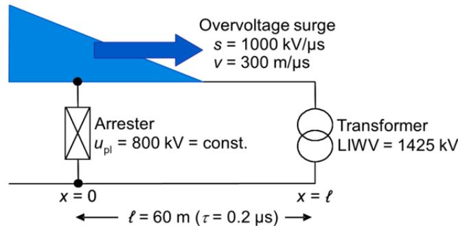
**Fig. 5:** Simplified arrangement to illustrate the protective zone of an arrester (explanation see text)
