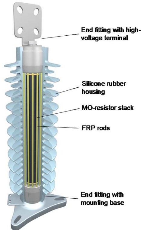
**Fig. 18:** Cross-sectional drawing of a polymer-housed MO high-voltage arrester of "cage design"
