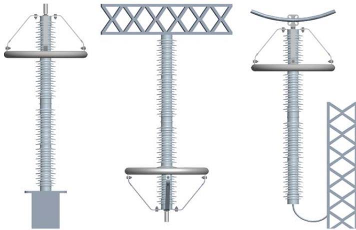
Position of the grading rings for different installations
