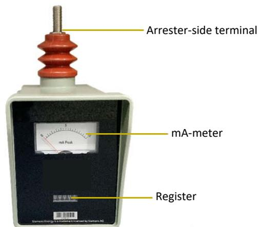
square value over a scaling factor is indicated. Most leakage current indicators are combined with a → [surge counter](#) in the same housing (see picture). Leakage current monitors are series-connected with the arrester in its earth connection. This requires installation of the arrester isolated from the ground by means of insulating feet (see [Figure 14](#)). Recent developments of leakage current monitors are based on the analysis of the third
