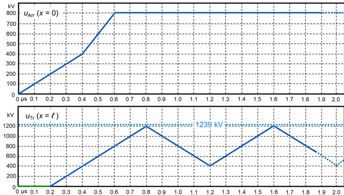
**Fig. 6:** Development of voltages at the arrester (top) and at the transformer (bottom)
