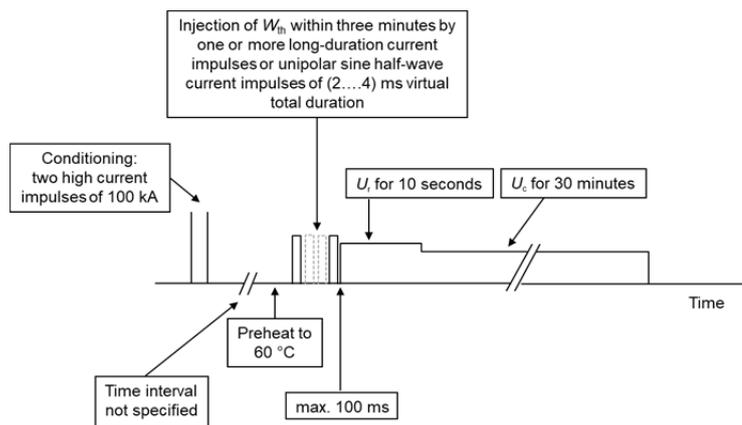
For [distribution class](#) (DL, DM, DH) arresters the test procedure looks different:
