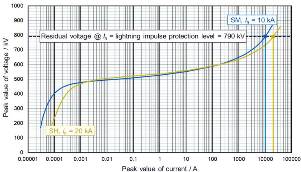
**Fig. 22:**  $U$ - $I$ -characteristics of two arresters of the same LIPL but different  $I_n$
