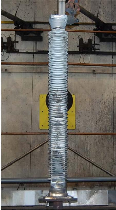
**Fig. 26:** Polymer-housed arrester ("tube design") after a test at rated short-circuit current (80 kA, 200 ms). The housing has remained completely intact.
