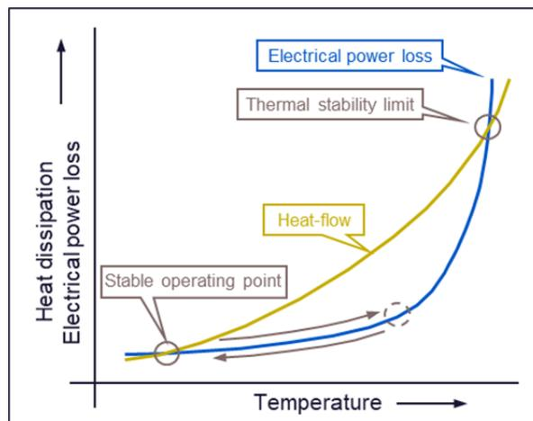
**Fig. 8:** Explanation of the thermal stability
