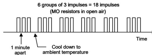
The test was considered passed if the resistors showed no evidence of puncture, flashover, cracking or other significant damage and their →[lightning impulse residual voltage](#) at →[nominal discharge current](#) had not changed by more than 5 %.
