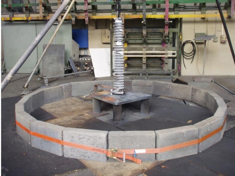
**Fig. 25:** Polymer-housed arrester ("cage-design") after a short-circuit test at rated current (65 kA, 200 ms). The housing is ripped but in mechanically sound condition. Details of the test setup can well be seen. For further information see [short-circuit tests](#) in the appendix.
