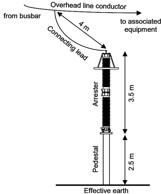
Fig. 7: Typical arrangement of an arrester in a 420 kV substation
