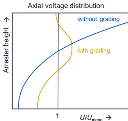
capacitances. The representation here shows the conditions in an outdoor arrester with and without a grading ring when using a purely capacitive equivalent circuit diagram as a basis. The vertical line shown for  $U/U_{mean} = 1$  corresponds to an ideal, uniform voltage distribution. However, because the MO resistors do not behave purely capacitively, but
