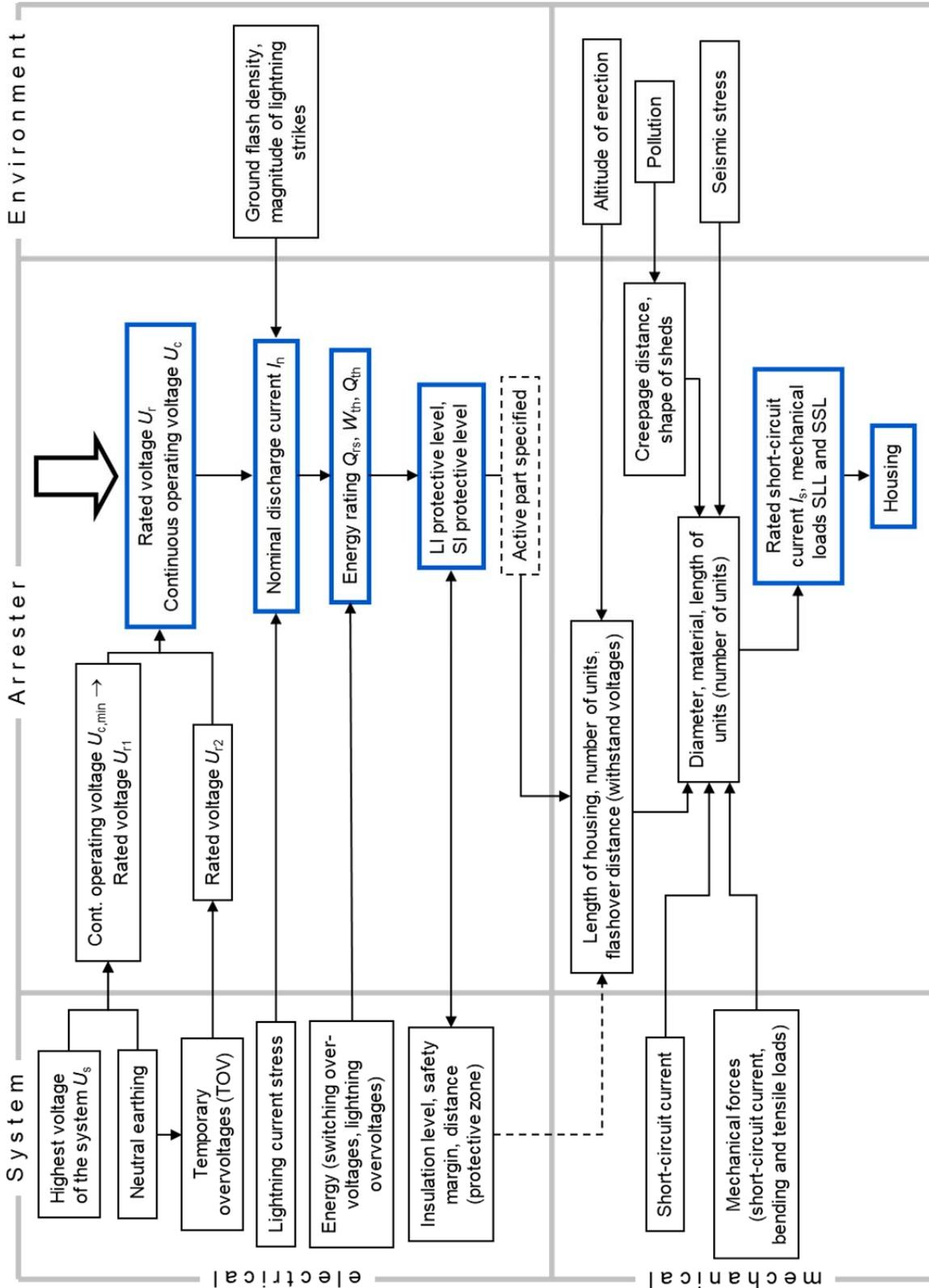
Fig. 20: Procedure for configuring an MO arrester
