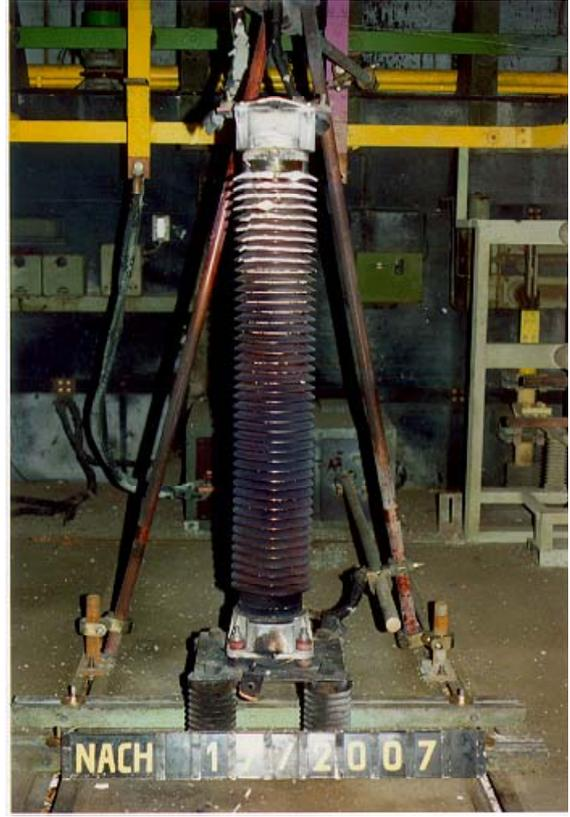
**Fig. 27:** Porcelain-housed arrester after a test at rated short-circuit current (63 kA, 200 ms). Apart from a few broken sheds, the housing has remained intact.
