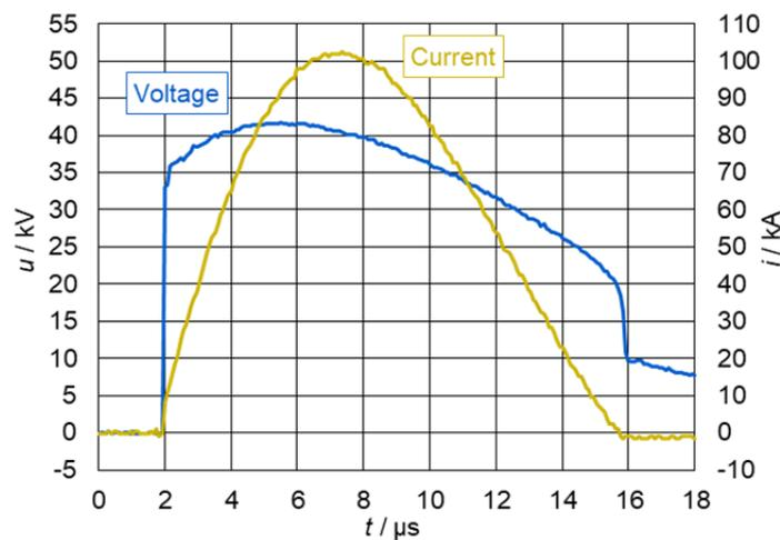
**High current impulse operating duty test:** this was a test in the former IEC 60099-4 Ed. 2.2, to be performed on distribution arresters and on the 20-kA High Lightning Duty arresters for the voltage range 1 kV to 52 kV. It had to be carried out on all arresters with → [nominal discharge current](#) of 1.5 kA, 2.5 kA or 5 kA and on arresters with nominal discharge current of 10 kA and → [line discharge class](#) 1. This test does not exist anymore in IEC 60099-4 Ed. 3.0.
