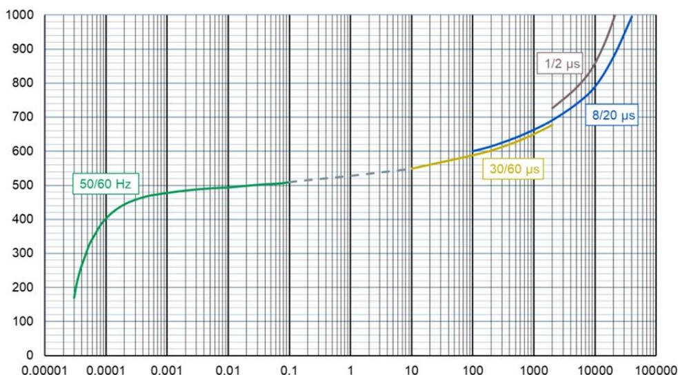
inductive component due to the arrester's self-inductance must be included in the characteristic curve for steep current impulses, which is why its actual course depends on the arrester length. The figure presented here shows an example of a complete characteristic curve, as shown only in simplified form in Figure 2.
