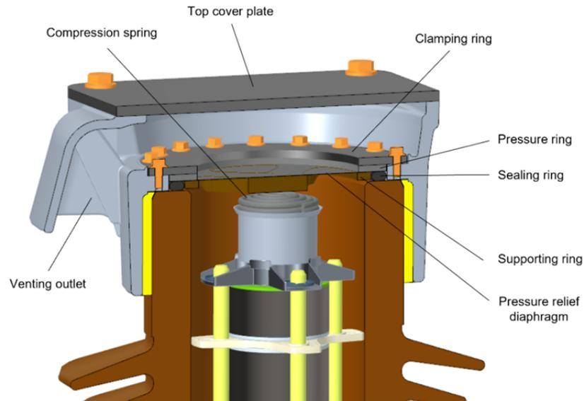
**Fig. 12:** Sealing system of a high-voltage porcelain housed MO
