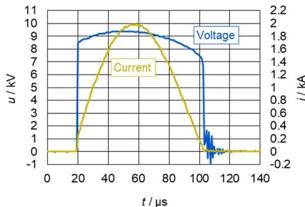
front time (IEC 60099-4 Ed. 3.0, 3.68). Switching current impulses are used in the laboratory to ascertain the →[voltage-current-characteristic](#) of arresters, →[arrester sections](#) or →[MO resistors](#). They are produced by a capacitor discharge in an aperiodically damped RLC circuit. The current amplitudes are within a range of 125 A to 2 kA. The oscillogram depicts an example of a residual voltage measurement on an MO resistor at a switching current impulse of 2 kA.
