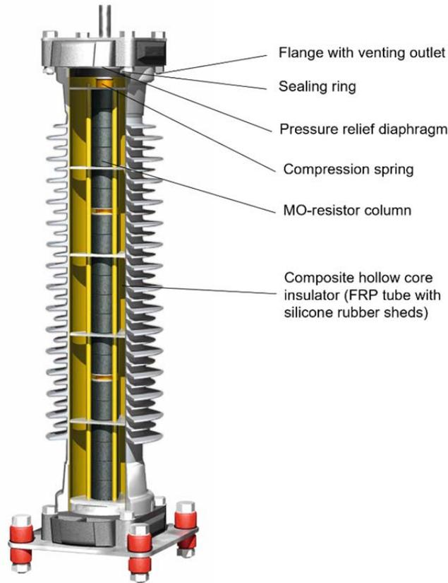
**Fig. 19:** Cross-sectional drawing of a polymer-housed high-voltage arrester of "tube design"
