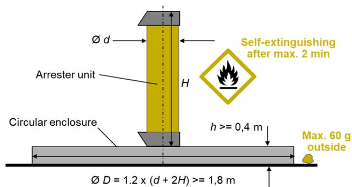
**Short-circuit withstand (capability):** ability of an arrester to withstand the short-circuit current that flows after an overload, without causing violent shattering of the housing. The short-circuit withstand capability used to be referred to as →[pressure relief class](#), and is now indicated as →[rated short-circuit current](#)  $I_s$  and proved by means of →[short-circuit tests](#).
