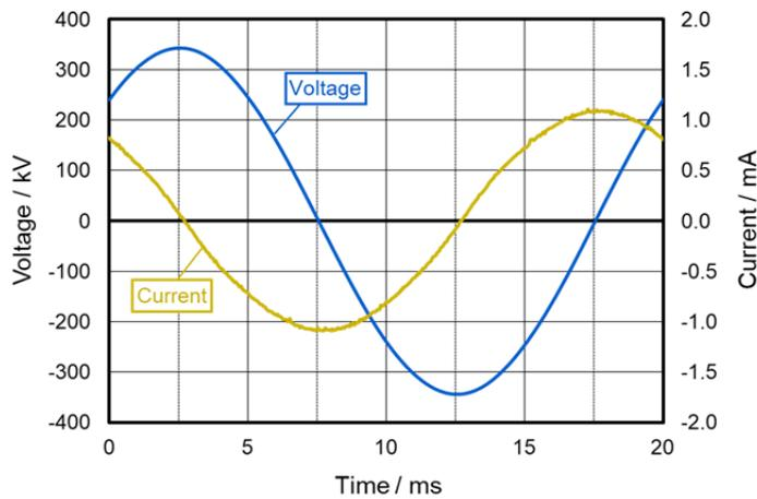
**Fig. 3:** Applied voltage and leakage current of the sample arrester of Fig. 2 when operated at phase-to-earth voltage ( $U_s = 420 \text{ kV}$ ,  $U_r = 336 \text{ kV}$ )
