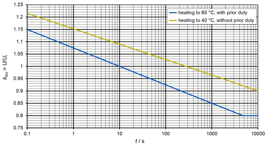
Fig. 21: Example of a power-frequency voltage versus time ( $U-t$ ) characteristic
